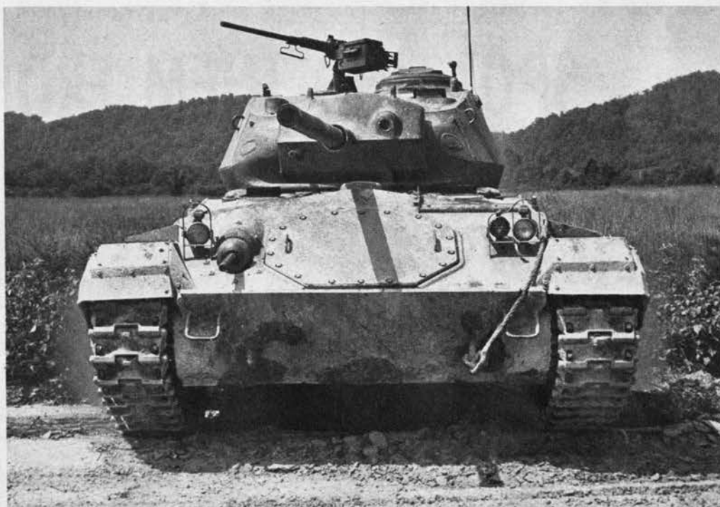
AA weapon on the M-24 is set at right (see silhouette) and cupola is at the extreme left atop the turret. With low silhouette and gun extending forward, the M-24 resembles Russian T-34.
